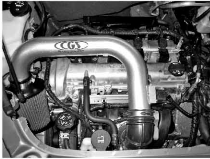
[Completed installation shown on 2006 Chevy HHR with 2.4L engine.]
